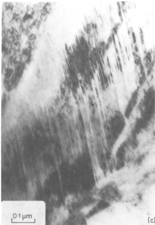
Figure 1 As-quenched optical microstructures of (a) CW and (b) PM high-speed steels, and (c) electron micrograph of internal twinning within martensite.
